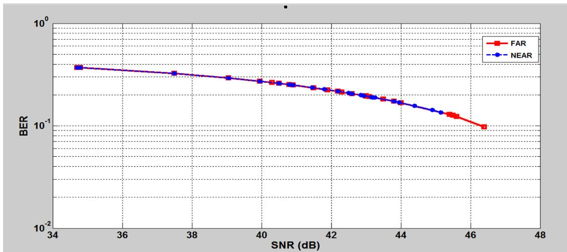
Figure 7: Comparison of BER Performance for Bluetooth Interference (Near and Far)
