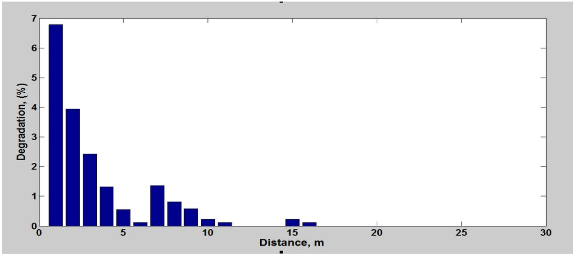
Figure 6: Comparison of SNR Degradation for Bluetooth Interference (Near and Far positions)
