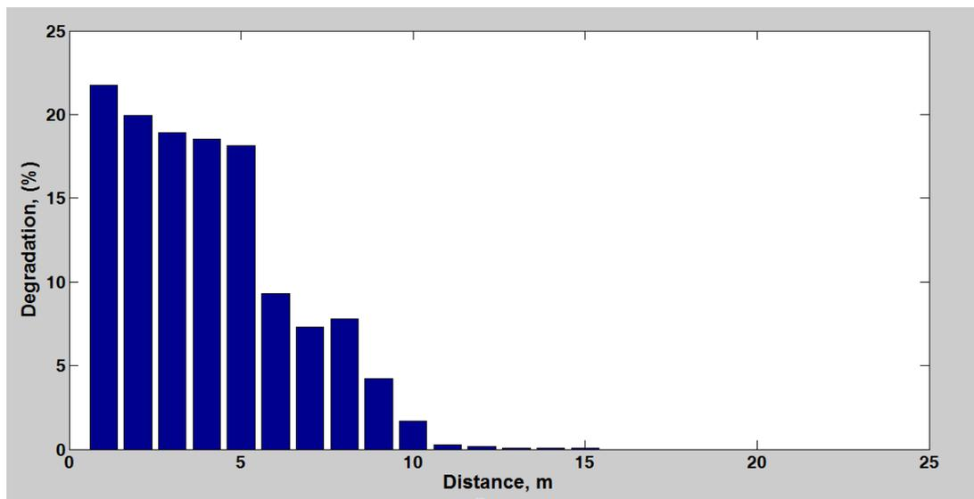
Figure 5: Comparison of RSS Degradation for Bluetooth Interference (Near and Far Positions)
