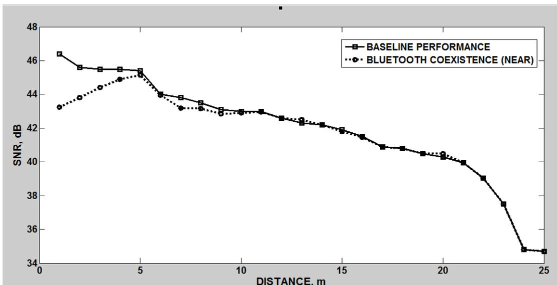
Figure 4: Comparison of Baseline Performance with Bluetooth Interference (SNR vs Distance)
