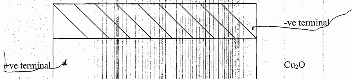
Fig. 3: Completed backwall solar cell
