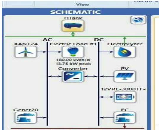
Figure 3: Systematic diagram of how hybrid energy is been configured
