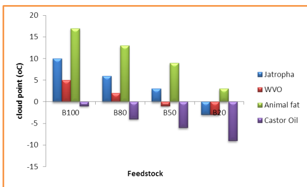
Fig. 5: Variation of Cloud point for different feedstocks
