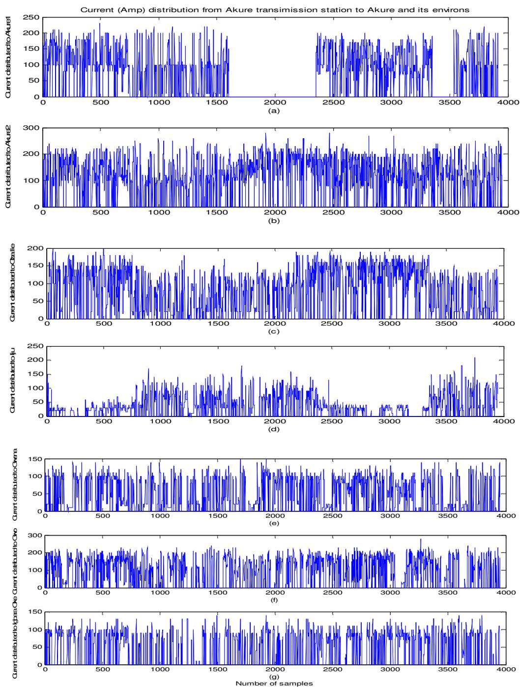
Fig. 3: Graph of total power in terms of current distributed from the 132kV Omotosho transmission station in Akure to: (a) T2B\_Akure, (b) T2C\_Akure, (c) Oba\_Ile, (d) Iju, (e) Owena, (f) Owo and (g) Igbara\_Oke.
