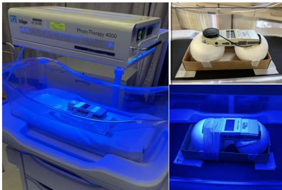
Figure 1: An irradiance meter is mounted on a foam platform to simulate a newborn head. The Dräger Phototherapy 4000 lamp was used at varied distances to achieve different irradiance levels (left). The newborn head model is shown without phototherapy (top right) and with phototherapy and sock top shield (bottom right).
