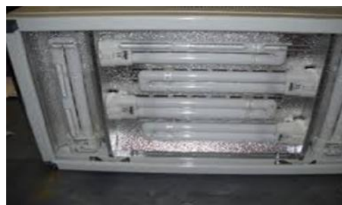
Fig 1; Locally fabricated (F) phototherapy devices F 1- 4 and a commercially-obtained (C) device. F1, 2, and C use fluorescent lamps, while F3 and 4 use led-tubes as light sources.
