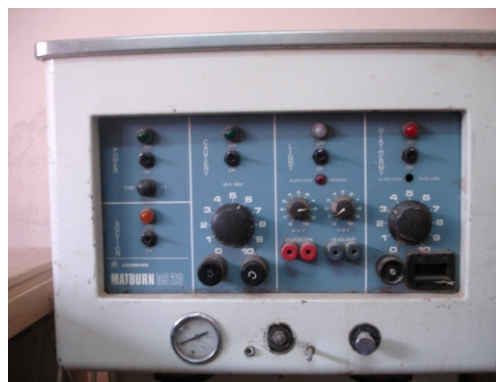
Fig 1: Old diathermy machine that uses spark gap principle
