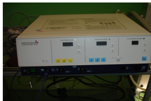
Fig 2 Recent model of diathermy machine that uses valve oscillators
