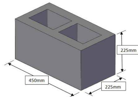
Figure 2: Standard size of a sandcrete block
