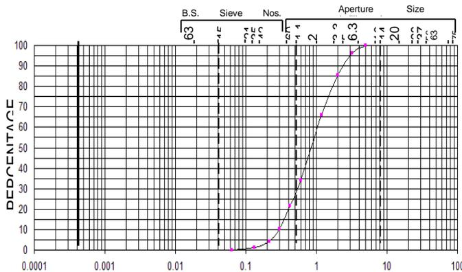
Figure 1 Particle size analysis of the sand
