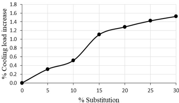
Figure 7. Changes in building cooling load with metakaolin substitution
