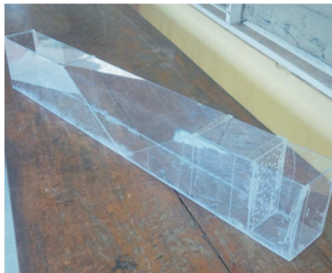
Plate 1: V-notch side weir of no sill height
