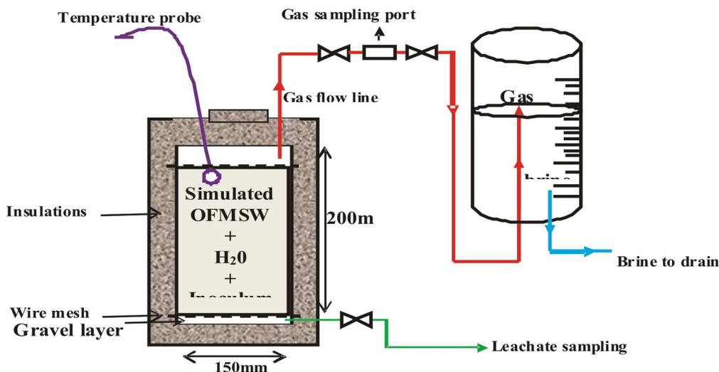
Figure 1: Experimental set-up adapted and modified from West *et al.* (1998)
