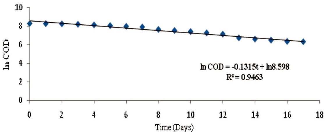
Figure 6: Testing fenton's first order kinetics for OFMSW/CD
