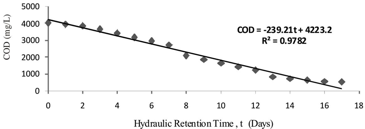
Figure 4: Testing zero order kinetics for COD (OFMSW with CD)
