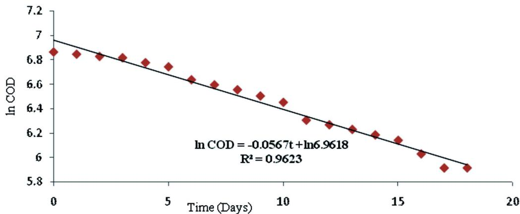
Figure 7: Testing fenton’s first order kinetics for OFMSW
