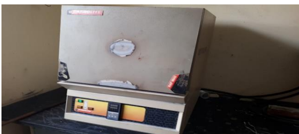
Plate 2: Carbolite incinerator/oven used to burn the husk
