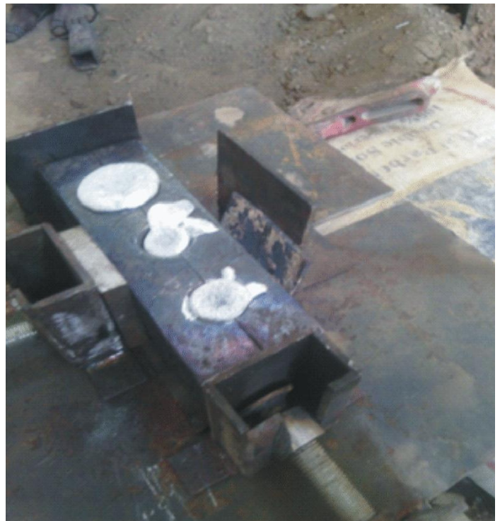
(b) A metal mould with the solidified alloy after vibration
