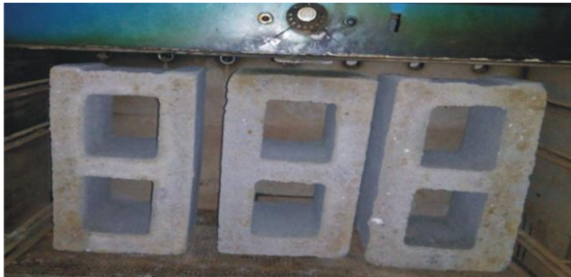
Plate 2: Block samples oven dry in oven for 24 hours
