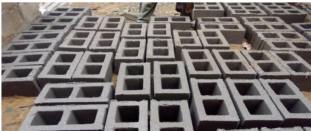
Plate 1: Metakaolin sandcrete blocks produced at various replacement levels
