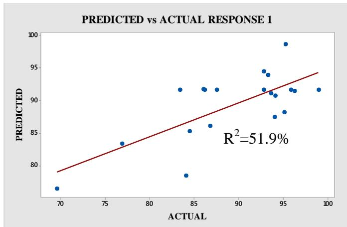
Figure 3: predicted versus actual plot for removal efficiency of Pb
