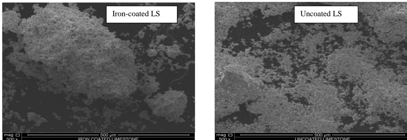
Plate 1: SEM image of iron-coated and uncoated limestone at x500 magnification
