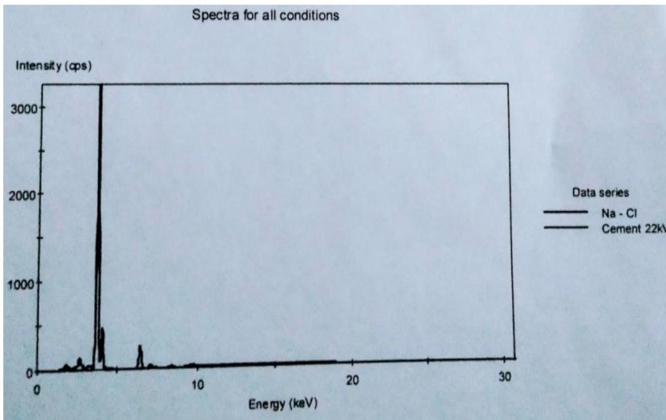
Figure 2: XRF graph of iron-coated limestone
