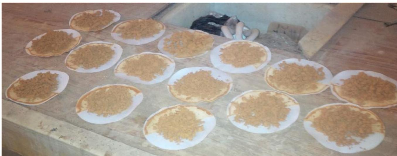
Figure 1: Air dried iron-coated limestone
