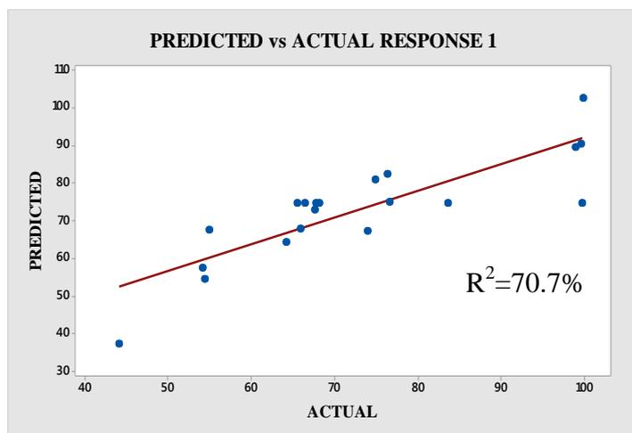
Figure 4: Predicted vs actual plot of removal efficiency for Cr.
