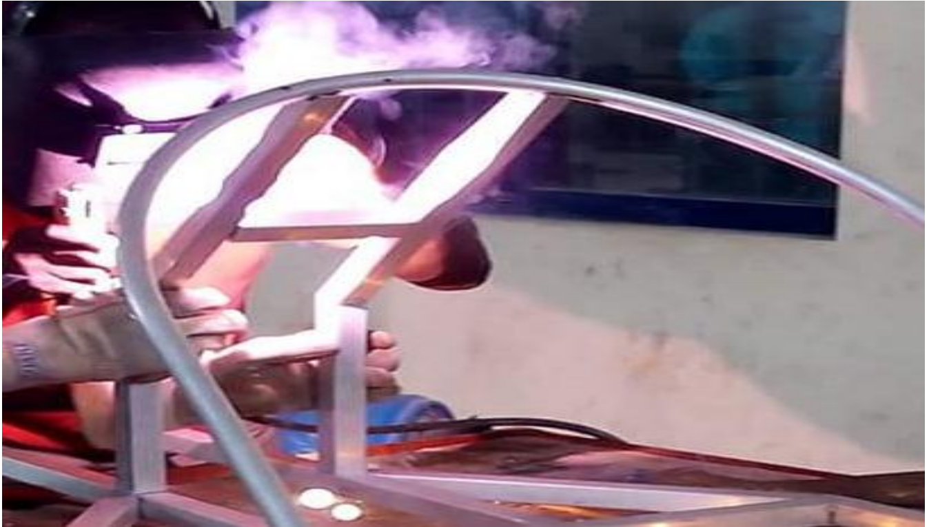
Figure 10: Chassis during fabrication
