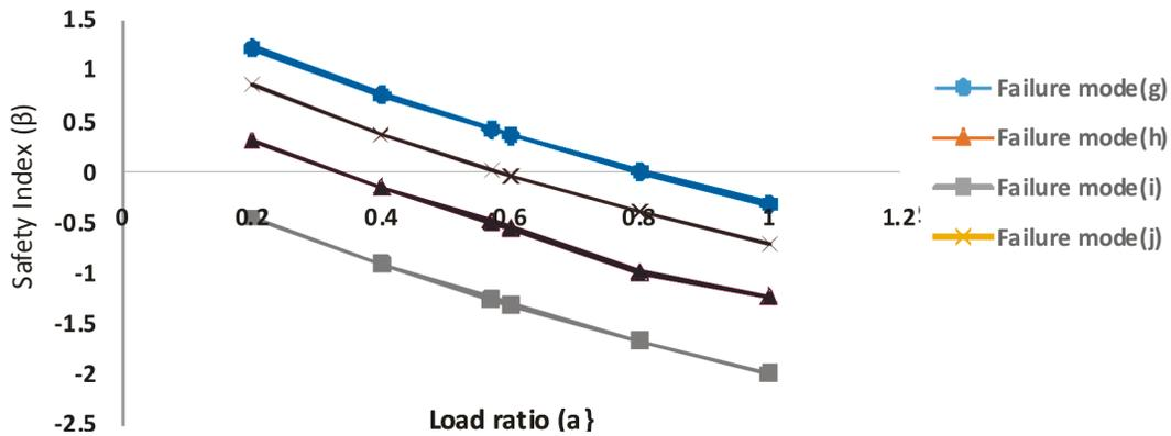
Figure 4: Safety level variations of the apex joint failure modes
