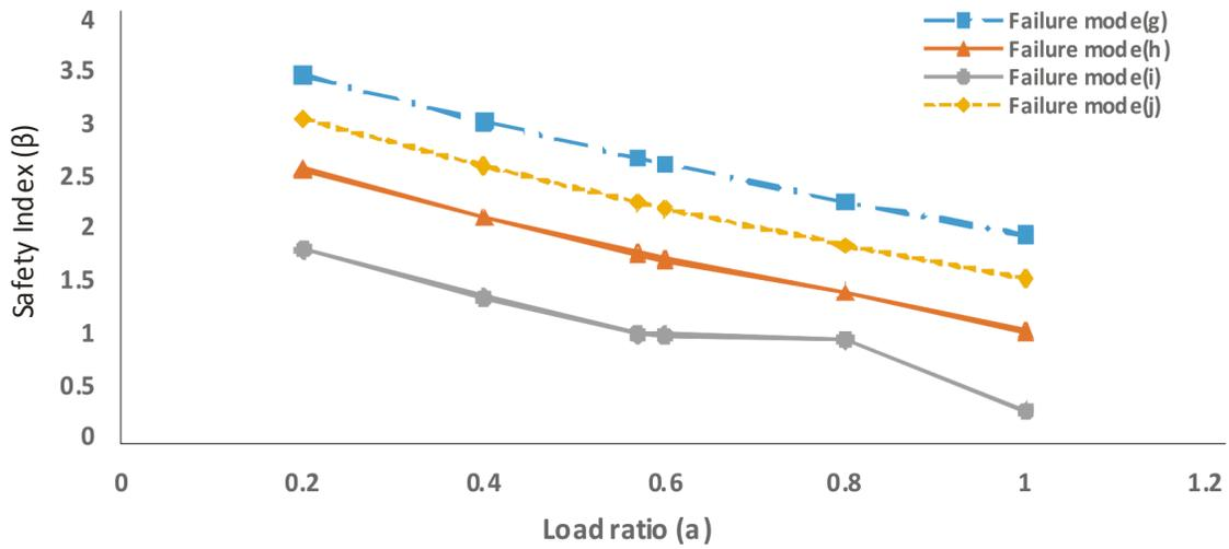
Figure 3: Safety level variations of the eaves joint failure modes
