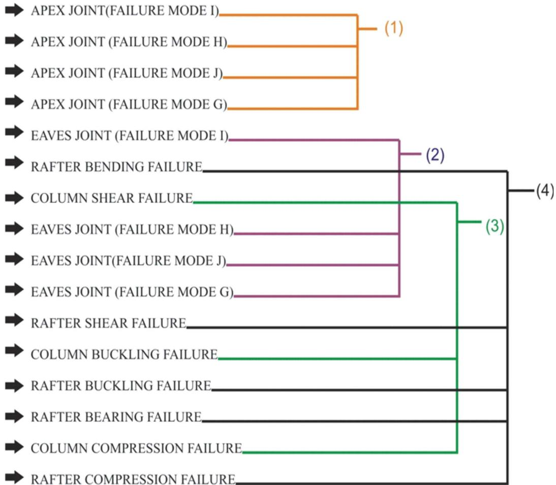
Figure 5: Sequence of failures for the portal frame at a design load ratio  $\alpha = 0.57$
