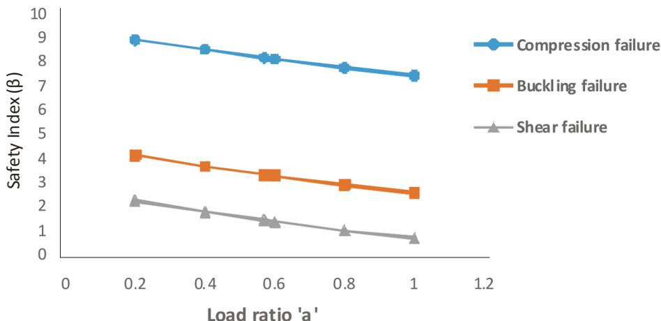
Figure 1: Safety level variations for column member failure modes
