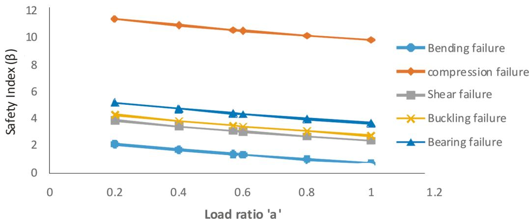
Figure 2: Safety level variation of the rafter member failure modes
