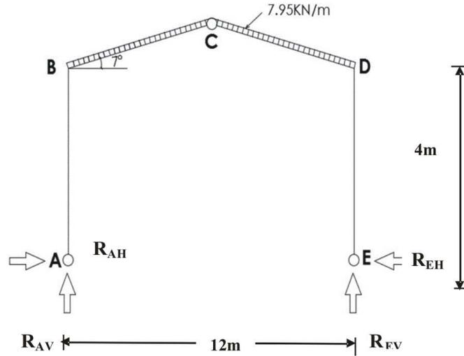
Figure 2: Idealized portal frame with reactive forces
