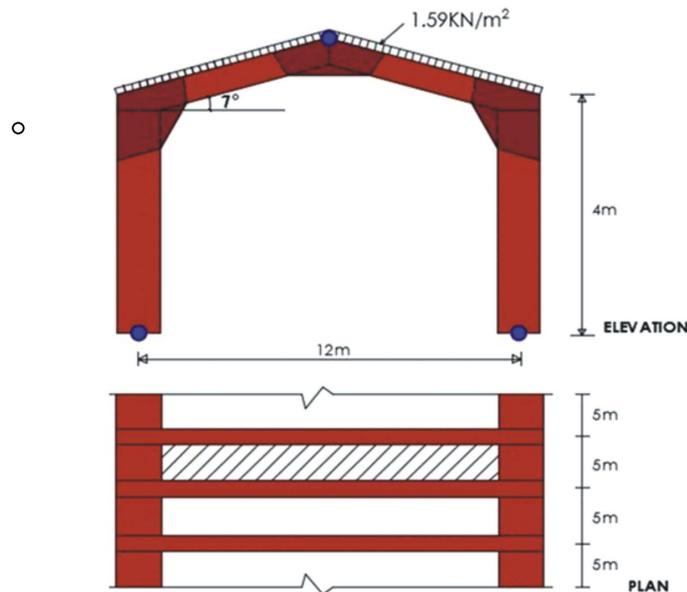
Figure.1: The plan and elevation views of the portal frame under investigation
