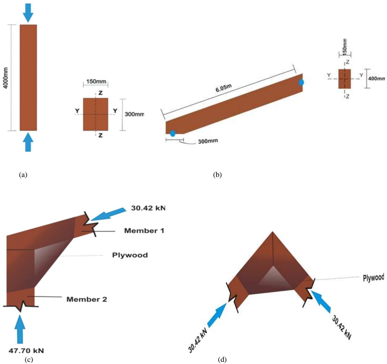
Figure 2: Details of portal frame showing (a) Column, (b) Rafter, (c) Eaves and (d) Apex
