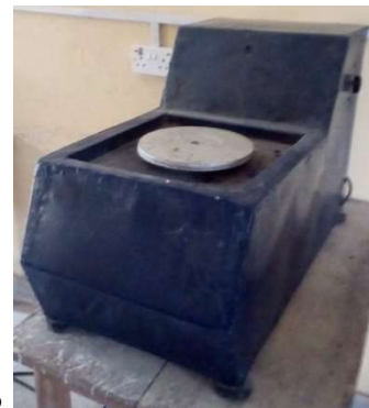
Figure 9: The 3D views (a,b) of complete laboratory polishing machine
