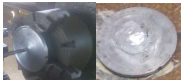
Figure 3: (a, b) cast aluminium alloy rotating disc machined on the lathe disc
