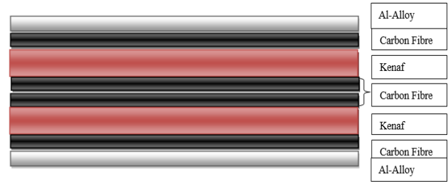
(b) Carbon Fibre Kenaf Reinforced Aluminium Laminate Figure 1: Composites Arrangement
