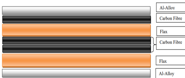
(a) Carbon Fibre Flax Reinforced Aluminium laminate
