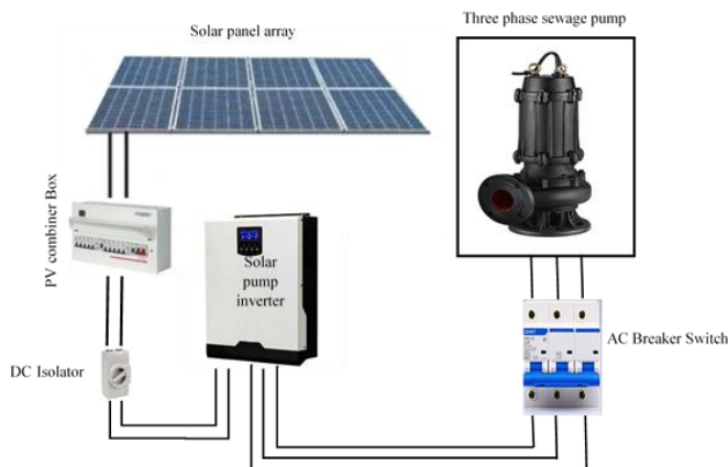
Figure 3. The proposed block diagram of the hybrid system
