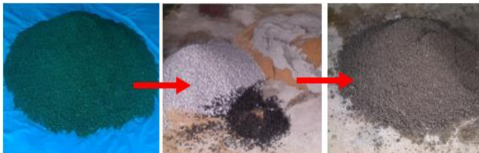
Figure 2: Material for Crumb-Rubber Masonry Concrete
