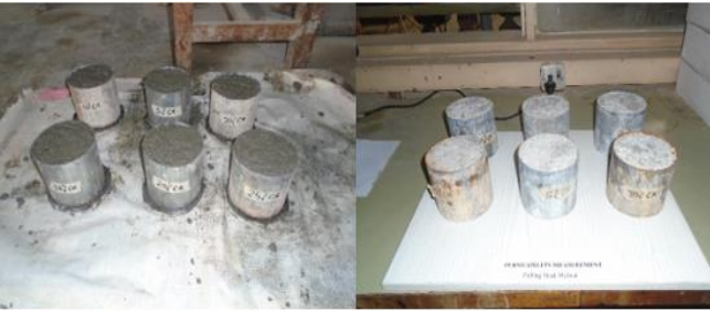
Figure 4: Masonry Concrete Samples for Water Permeability Test
