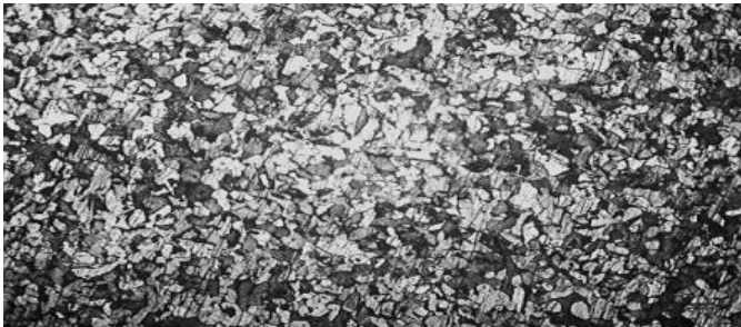
Figure 8b Microstructure of sample showing HAZ at welding current of 213A
