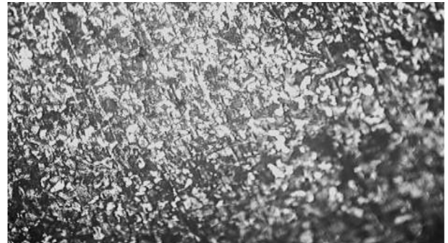
Figure 6b: Microstructure of sample showing HAZ at welding current of 155A
