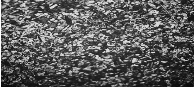
Figure 7b: Microstructure of sample showing HAZ at welding current of 190A
