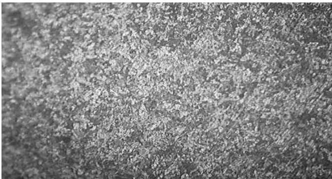
Figure 5a: Microstructure of sample showing fusion zone at welding current of 120A
