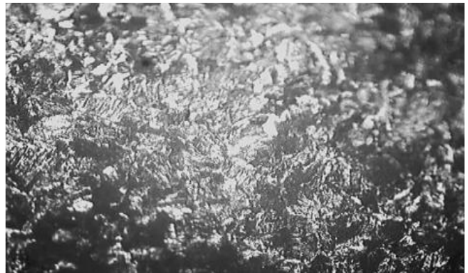
Figure 6a: Microstructure of sample showing fusion zones at welding current of 155A
