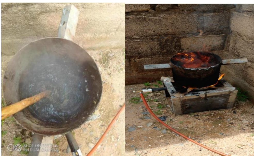
Plates 1a & 1b: Melting of the plastic waste
