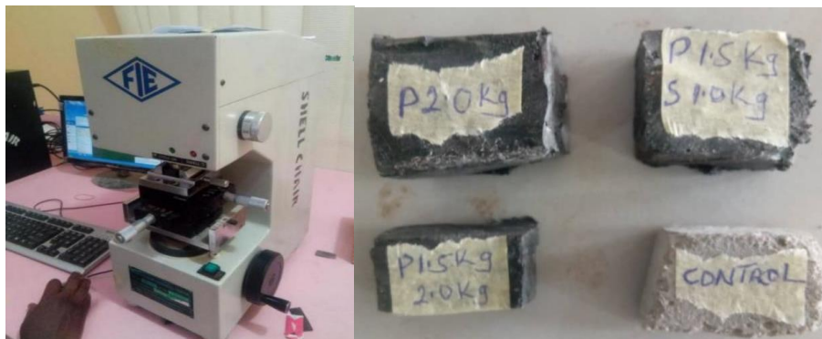
Plate 5a: Vickers Testing Machine Plate 5b: Composite Sample for Hardness Test
