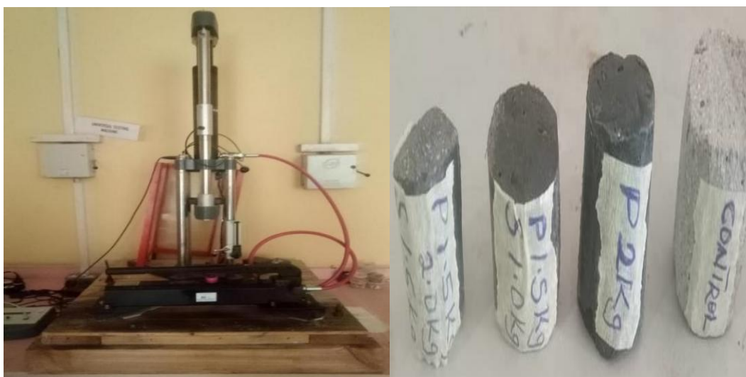
Plate 4a: Universal Testing Machine Plate 4b: Composite sample for Compressive strength test
