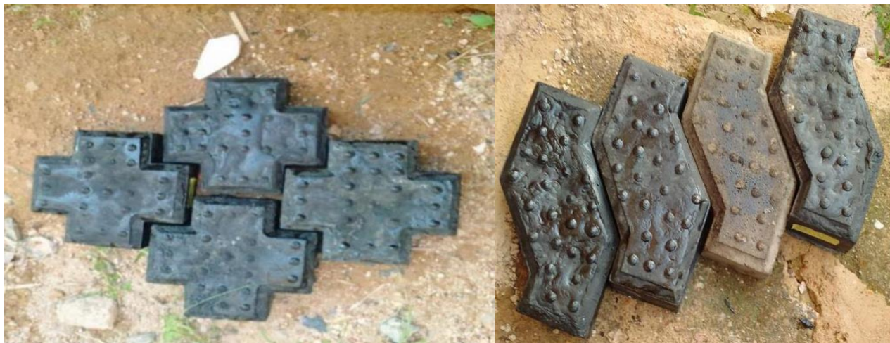
Plates 3a &amp; 3b: Developed plastic pavement block composites
