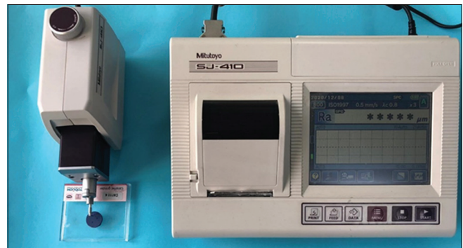
Figure 2: Surface Roughness Measurement Device (Mitutoyo Corp., Japan) and Sample Surface Tested at Three Different Points
