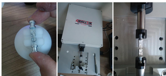
Figure 2: Placing the samples prepared in the study in a microtensile testing machine
