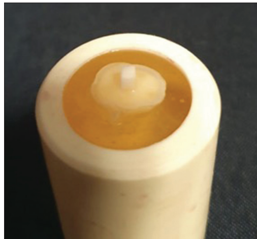
Figure 2: The view of the zirconia specimens bonded to the dentin specimens by cement
