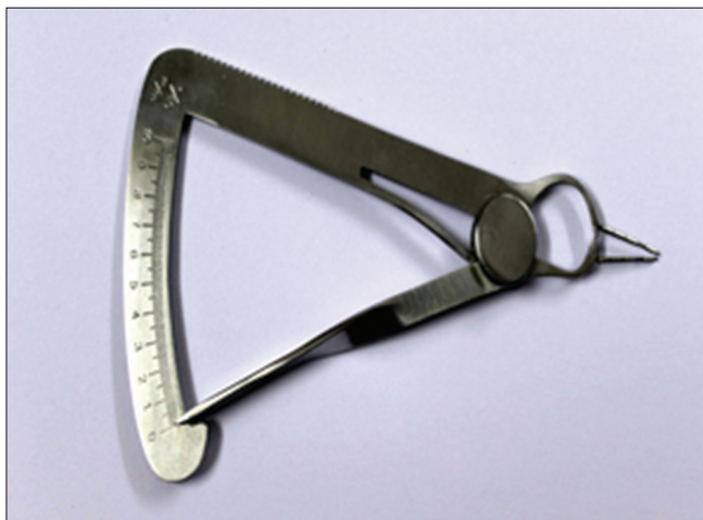
Figure 3: Modified caliper with periodontal probe attachments
