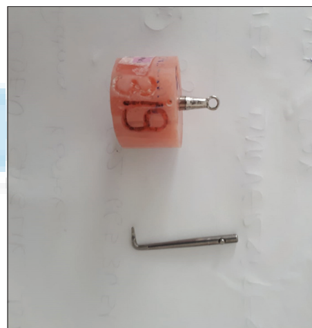
Figure 2: The specimen were embedded in self-curing acrylic resin
