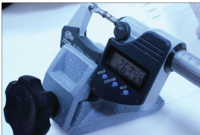
Figure 3: The first measurement of abutment coping complex without any cement inside
