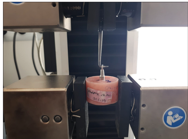
Figure 4: The pull-out test of the specimen in Instron machine
