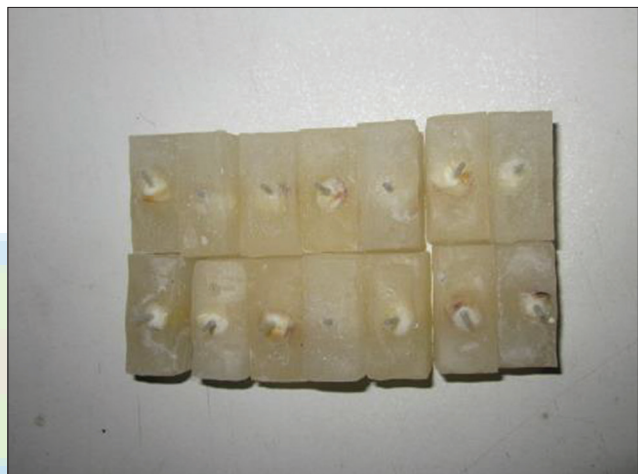
Figure 2: Samples on acrylic molds for push-out test
