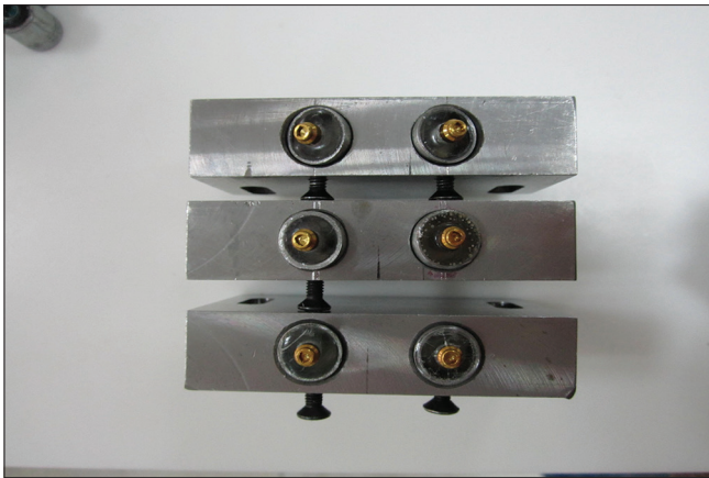
Figure 1: Three holder apparatuses with angles of 0°, 10°, and 20° to the x-axis
