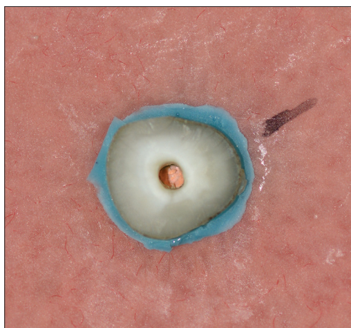
Figure 1: Specimen with standardized silicone layer, which simulated the periodontal ligament
