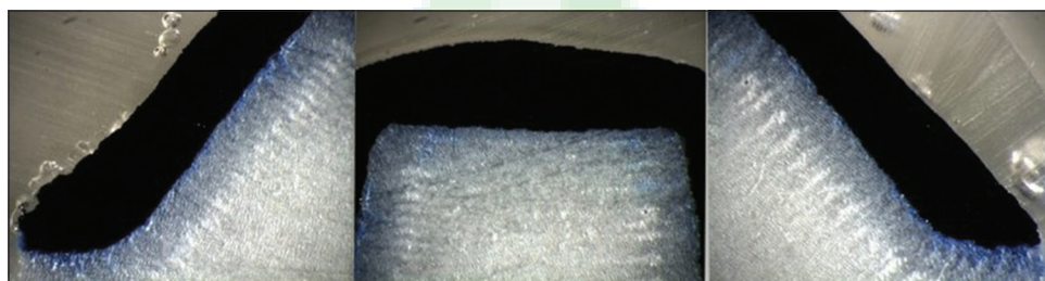
Figure 4: The sections of the cemented models were used to analyze the cement film thickness
