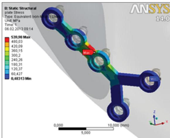
**Figure 7:** Three-dimensional Von Mises stress distribution fields in Y plate
