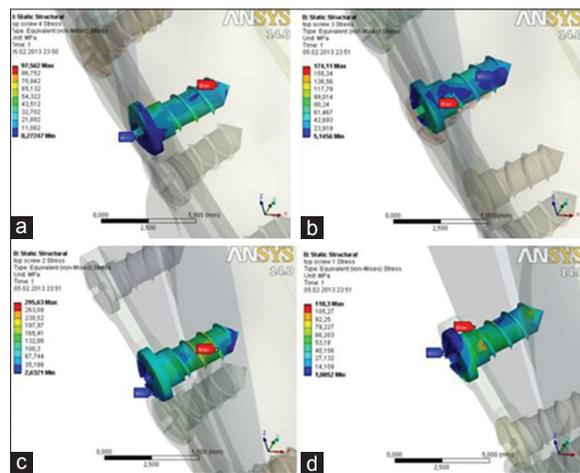
Figure 3: Three-dimensional Von Mises stress distribution fields in screws of upper plate, (a) 1<sup>st</sup> screw, (b) 2<sup>nd</sup> screw, (c) 3<sup>rd</sup> screw, (d) 4<sup>th</sup> screw
