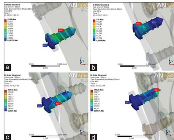
Figure 4: Three-dimensional Von Mises stress distribution fields in screws of lower plate, (a) 1<sup>st</sup> screw, (b) 2<sup>nd</sup> screw, (c) 3<sup>rd</sup> screw, (d) 4<sup>th</sup> screw
