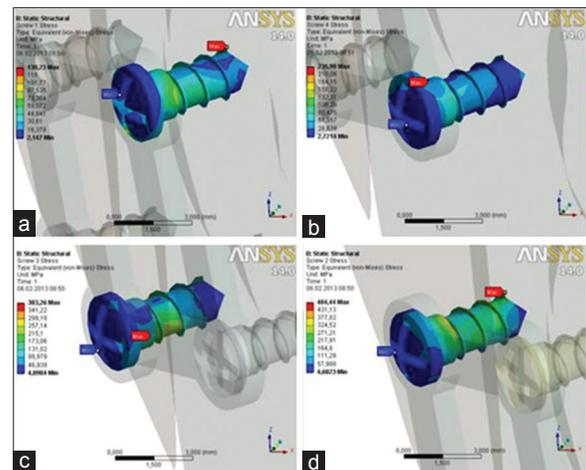
Figure 6: Three-dimensional Von Mises stress distribution fields in screws of square plate, (a) 1<sup>st</sup> screw, (b) 2<sup>nd</sup> screw, (c) 3<sup>rd</sup> screw, (d) 4<sup>th</sup> screw
