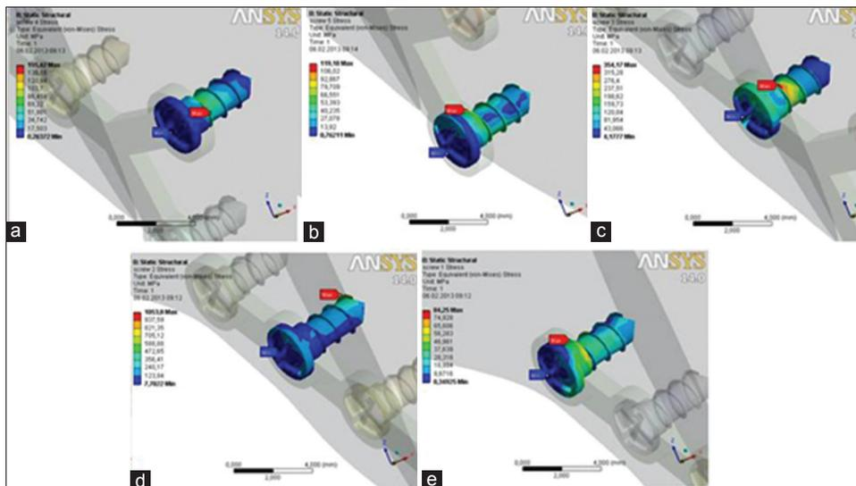
**Figure 8:** Three-dimensional Von Mises stress distribution fields in screws of Y plate, (a) 1<sup>st</sup> screw, (b) 2<sup>nd</sup> screw, (c) 3<sup>rd</sup> screw, (d) 4<sup>th</sup> screw, (e) 5<sup>th</sup> screw
