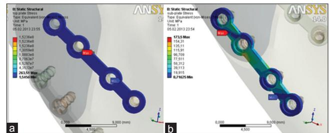
Figure 2: Three-dimensional Von Mises stress distribution fields in (a) upper and (b) lower straight plates
