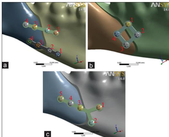
Figure 1: Three-dimensional finite element models: (a) Double straight plates, (b) Square plate, (c) Y plate
