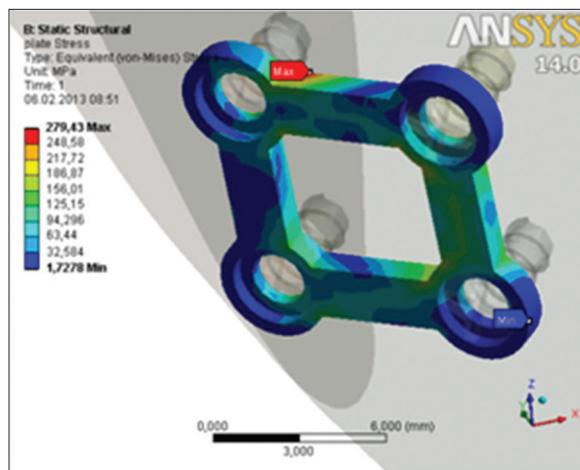
Figure 5: Three-dimensional Von Mises stress distribution fields in square plate
