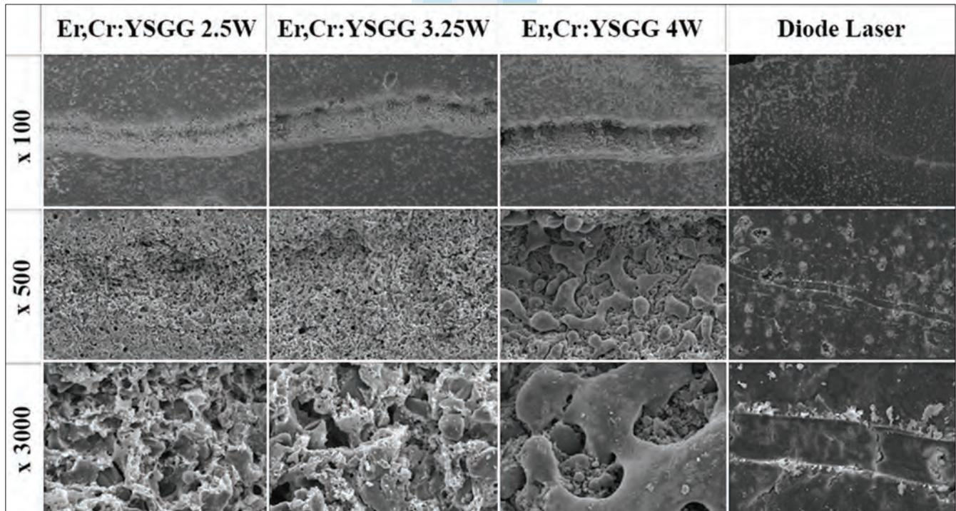
**Figure 4:** Scanning electron microscopy images of glass ionomer cement samples
