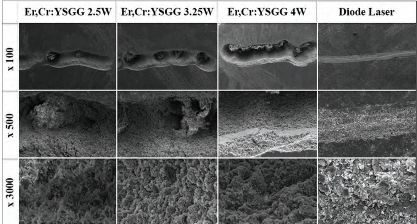
Figure 5: Scanning electron microscopy images of resin-modified glass ionomer cement samples
