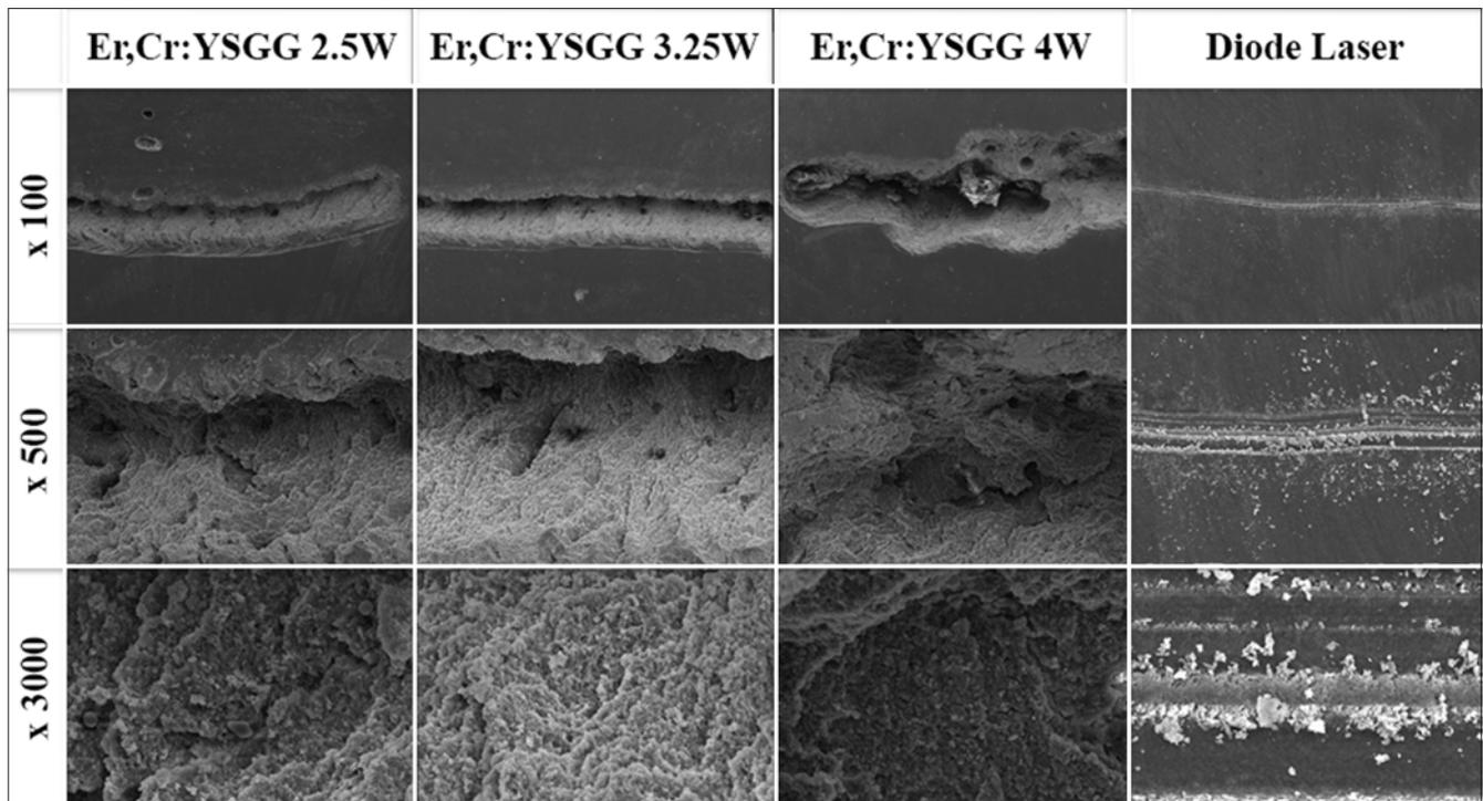
**Figure 3:** Scanning electron microscopy images of compomer samples
