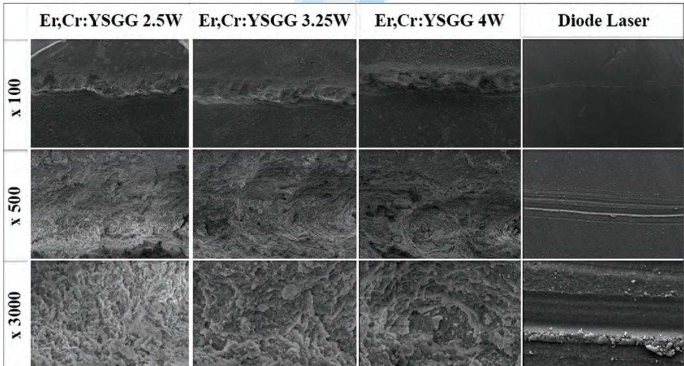
**Figure 2:** Scanning electron microscopy images of resin composite samples
