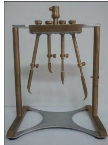
Figure 2: Measuring tool for anatomic points of knee. Relationship of the knee's anatomic points on paper. P: Centre of patella; T: Middle point of tuberositas tibiae ; L: Middle point of epicondylus lateralis ; M: Peak point of epicondylus medialis ; A: The point where the line combining peak points of epicondylus medialis and epicondylus lateralis intercepts with centre of patella in 90 degrees; B: The point where the line combining peak points of epicondylus medialis and epicondylus lateralis intercepts with middle point of tuberositas tibiae in 90 degrees
