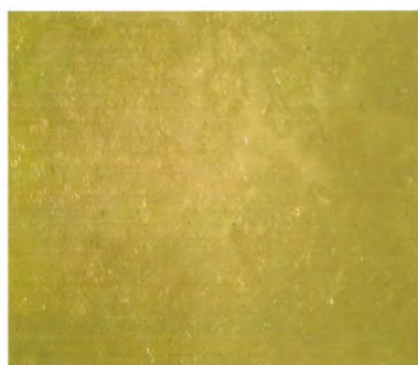
Fig. 2.0 Photomicrograph of 10%PS/90% PVAc blend without filler
