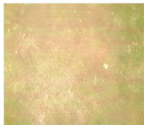
Fig. 2.15 Photomicrograph of 90%PS/10% PVAC blend without filler
