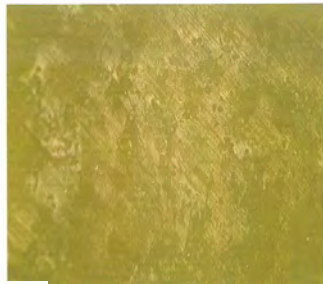
Fig. 2.6 Photomicrograph of 40%PS/60% PVAC blend with filler
