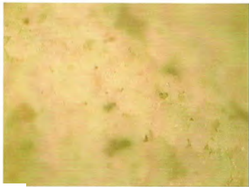
Fig. 2.5 Photomicrograph of 40%PS/60% PVAC blend without filler
