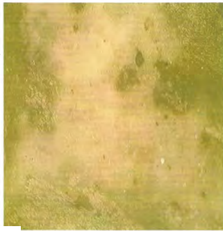
Fig. 2.13 Photomicrograph of 80%PS/20% PVAC blend without filler
