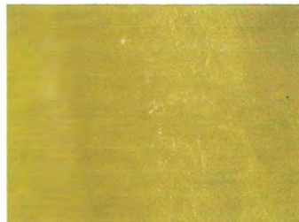
Fig. 2.19 Photomicrograph of 100% PVAC without filler
