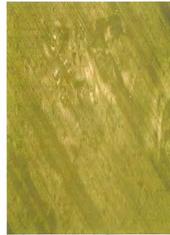
Fig. 2.16 Photomicrograph of 90%PS/10% PVAC blend with filler
