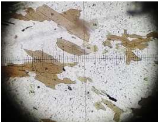
Figure 2: Biotite – muscovite schist showing a) in ppl biotite – Bt, plagioclase – Pl, muscovite – Ms and b) xpl granular, foliated fabric of the rock is presented.
