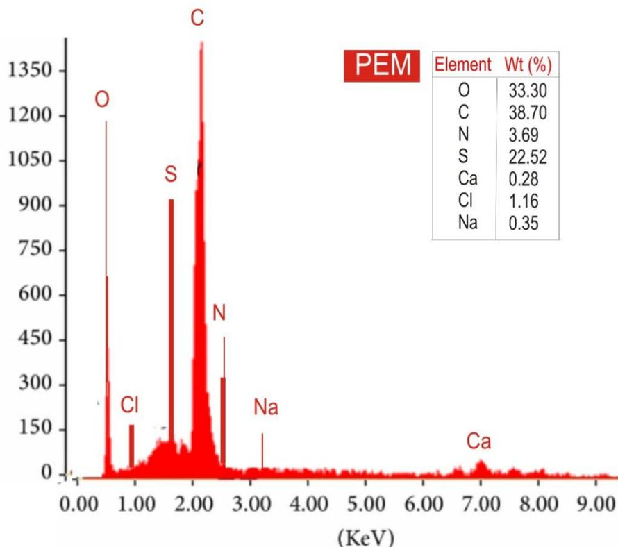
**Fig. 9:** The Energy Dispersed Spectroscopy (EDS) of Cation exchanged membrane
