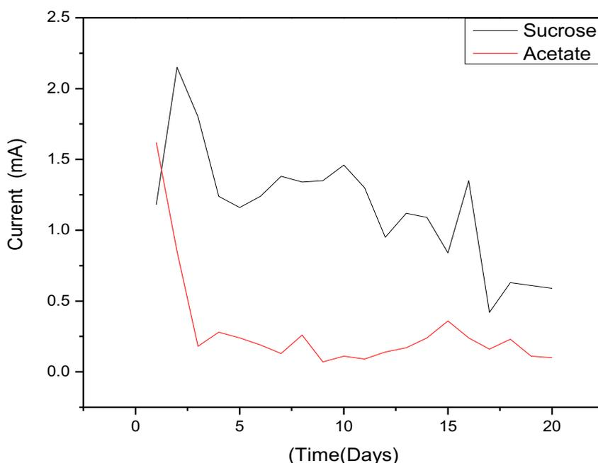
**Fig. 2:** Performance of bioelectricity generation using mixed culture in both sucrose and acetate carbon source enriched locust beans wastewater as substrate
