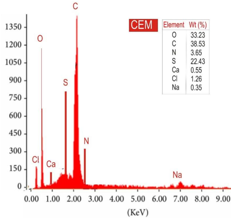
**Fig. 8:** The Energy Dispersed Spectroscopy (EDS) of Cation exchanged membrane
