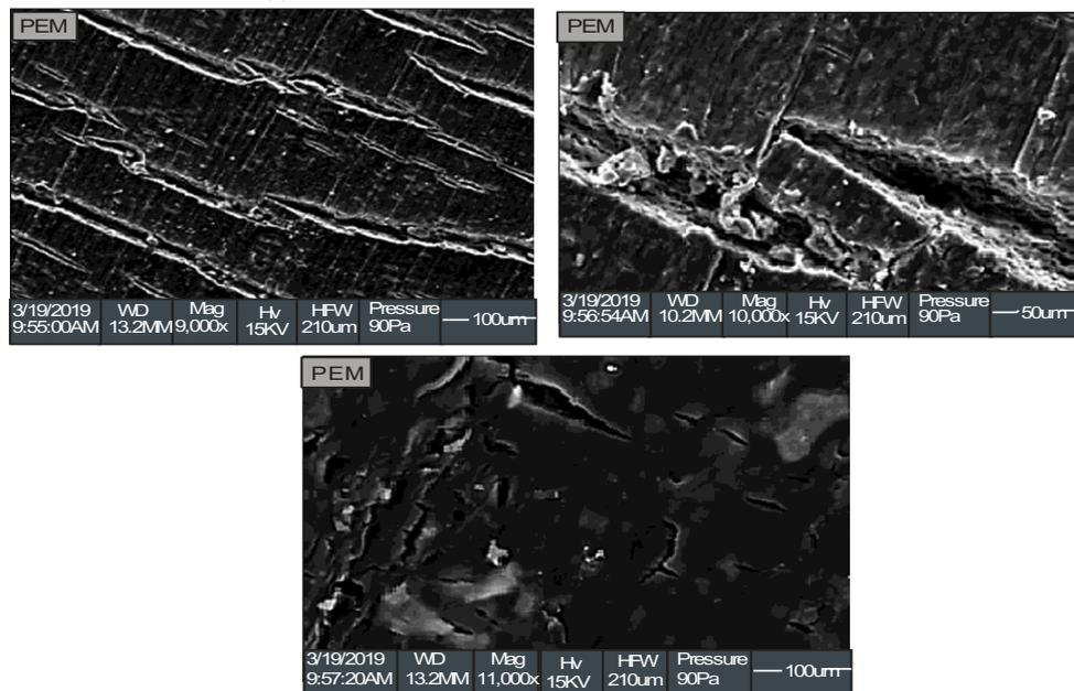
**Figure 7 -** Scanning electron microscope (SEM) image of cellulose acetate film membrane at 9000x, 10000x, and 11000x magnification
