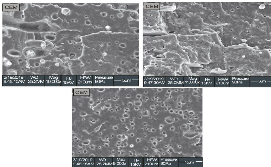
**Fig. 6:** Scanning electron microscope (SEM) image of cation exchange membrane at 9000x, 10000x and 11000x magnification
