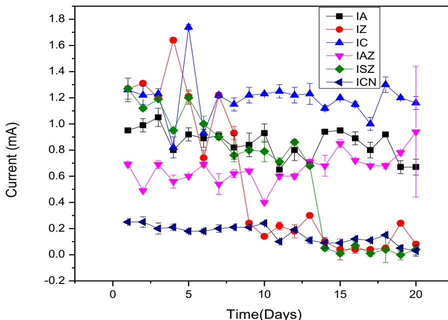
Figure 5: Graph showing the performance trend of different electrode material with *Myroides odoratimimus* (MO)
