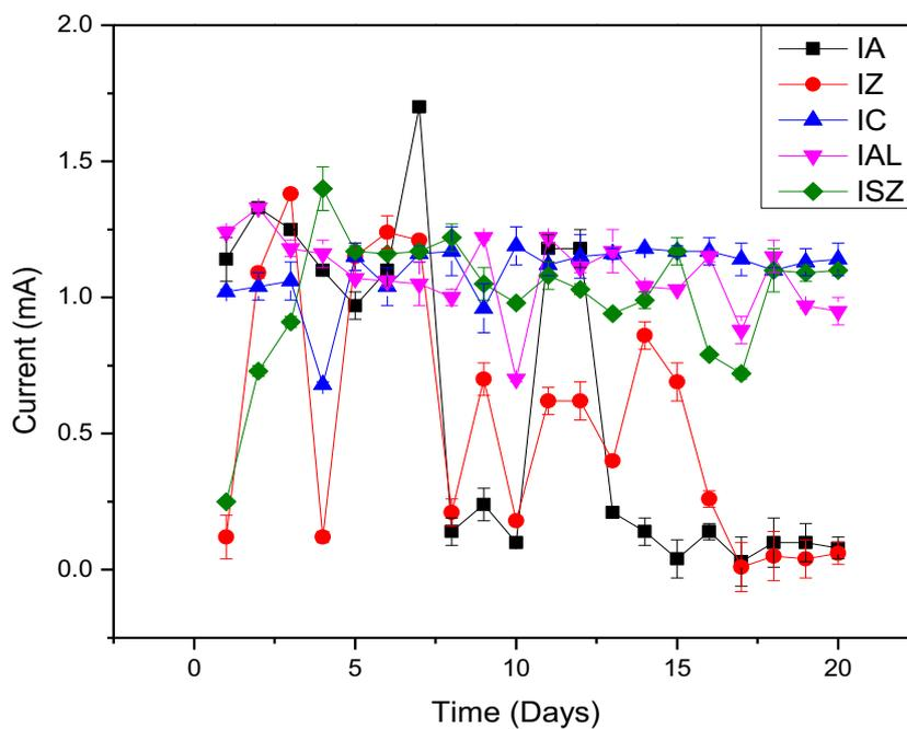
Fig. 4: Graph showing the performance trend of different electrode material with *Sphingobacterium mizutaii* (SM)
