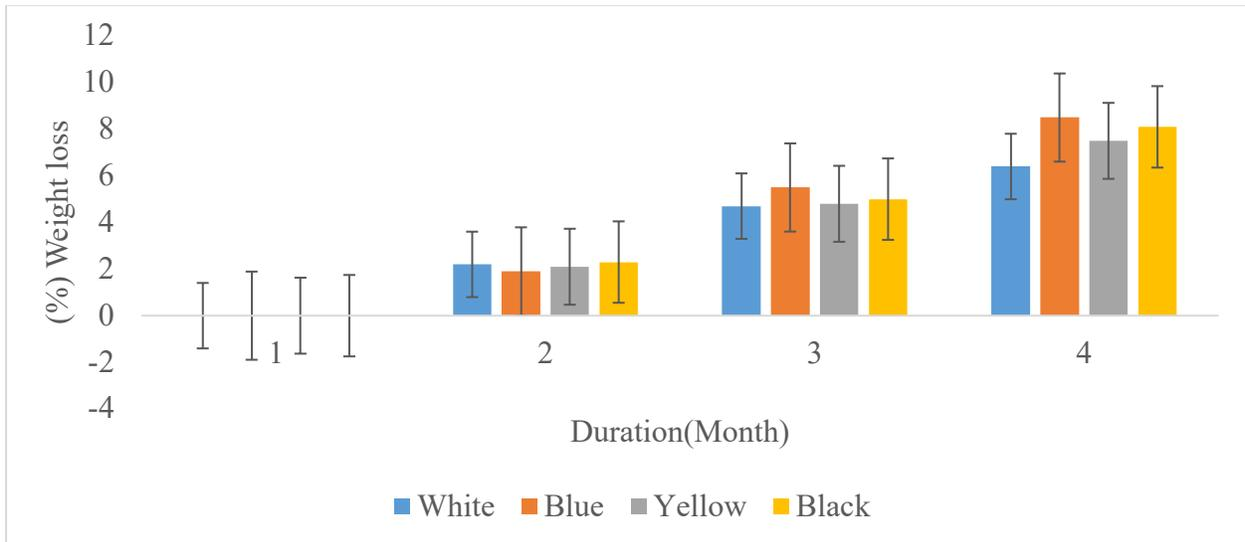
**Fig. 8:** Percentage (%) weight loss observed in all nylon samples during biodegradation for Site 2
