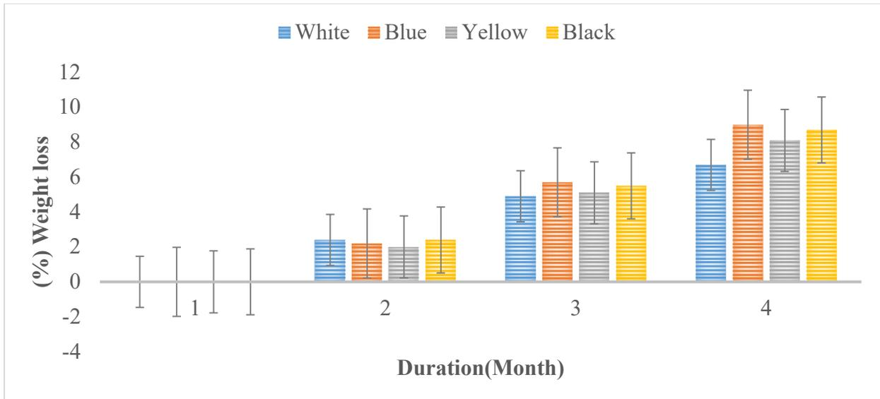
**Fig. 7:** Percentage (%) weight loss observed in all nylon samples during biodegradation for Site 1
