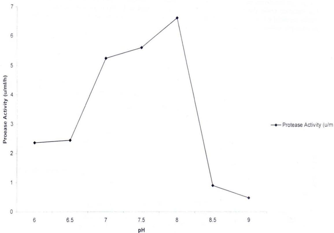
**Figure 2: Effect of pH on production of the protease of *S. thermovulgaris* at 50 °C for 96 h**
