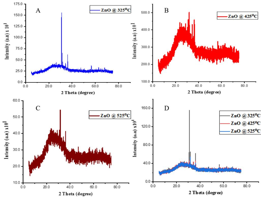
Fig. 1: X-ray diffraction spectra pattern of ZnO annealed at (a) 325 °C (b) 425 °C, (c) 525 °C and (d) combined spectra annealed at substrate temperature
