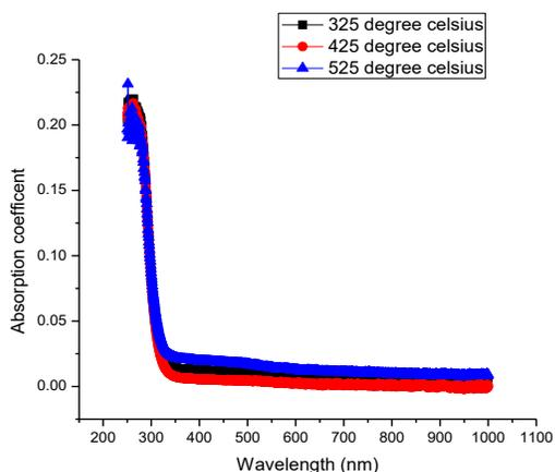
Fig. 4: Optical absorption coefficient of zinc oxide thin film
