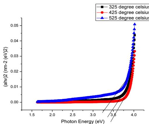
Fig. 5: Tauc plot of band gap energy of ZnO
