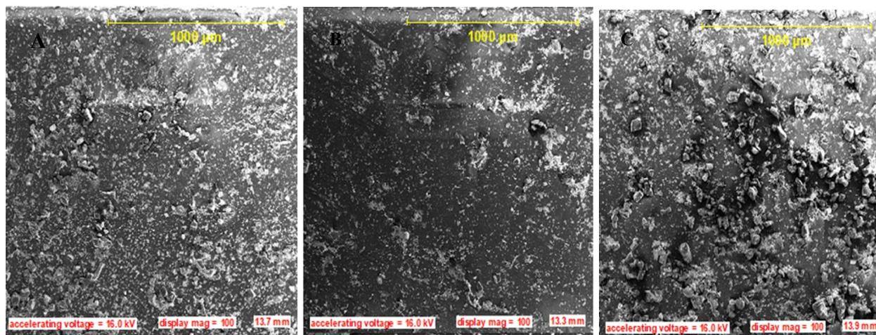
Fig. 6: Surface morphology images of ZnO thin film annealed (a, left) 325 °C, (b, middle) 425 °C, and (c, right) 525 °C
