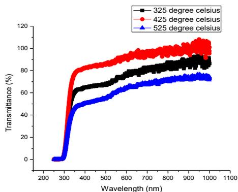
Fig. 2: Optical transmittance of ZnO thin film annealed at (a) 325 °C, (b) 425 °C and (c) 525 °C.
