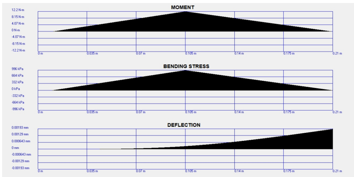
Fig.3: Effects of the moment, bending stress and the deflection on the auger shaft
