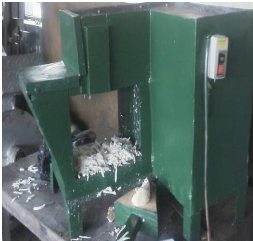
Plate 1: A photograph of the developed cassava slicing machine
