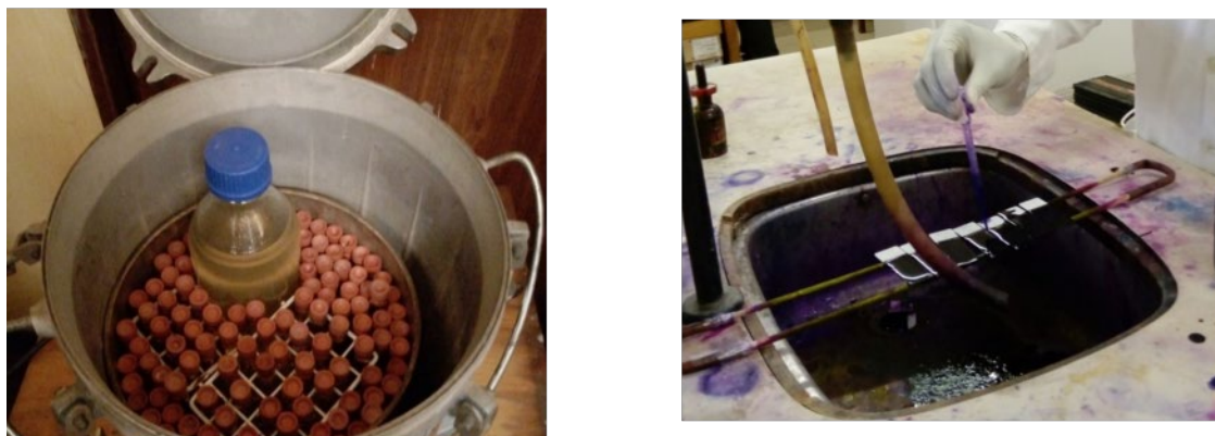
Figure 8: (a) Autoclaving process of diluent and media after Aga preparation and (b) Gram staining process
