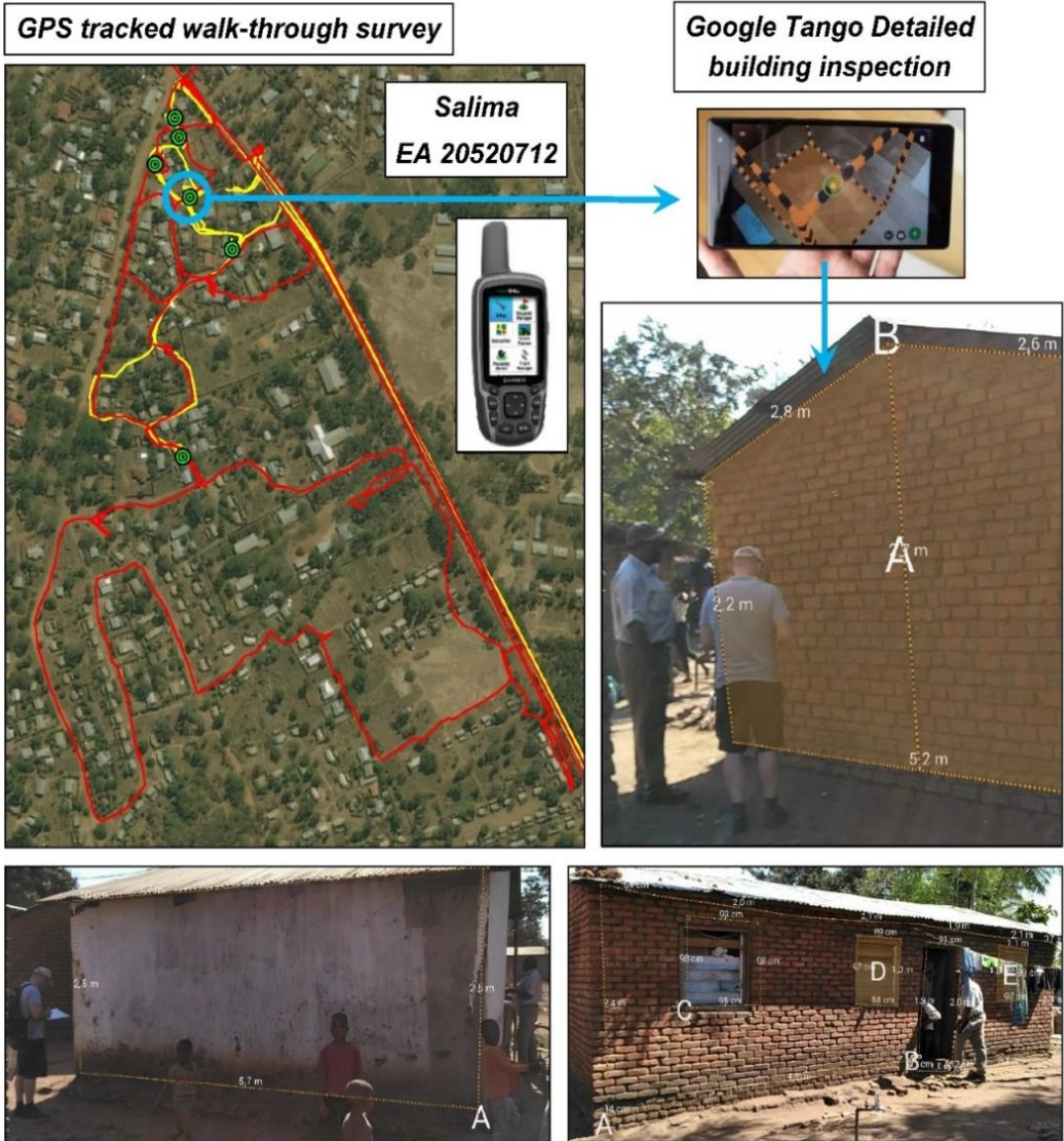
Figure 2: Quick walk-through and detailed building inspections in Salima EA20520712.
