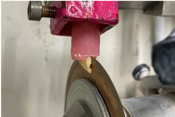
Fig. 1. Sectioning using the isomet into two halves in a buccolingual plane.
