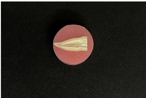
Fig. 2. Sectioned half of the root was embedded in self-curing resin with their dentine surface upward.
