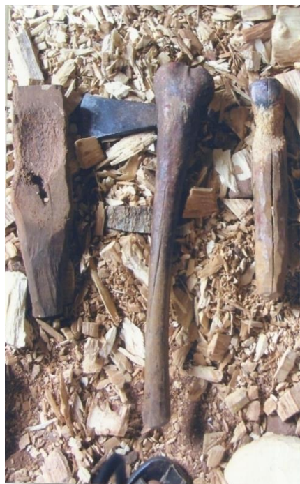
Anyu Ike & Utu (Axe and Mallet) Local Carving tools [©Researcher Arua J.E., 2016]
