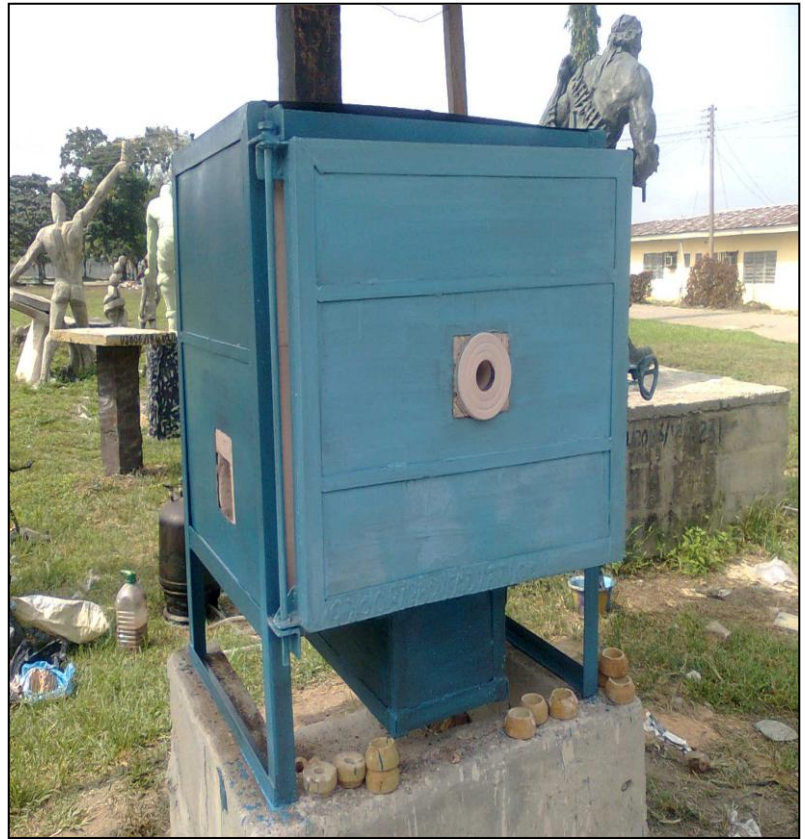
Plate 8. An Oil-Burning Kiln Constructed Entirely with Insulating Bricks, and Installed at the Department of Fine Arts And Design, In the University Of Port Harcourt.
