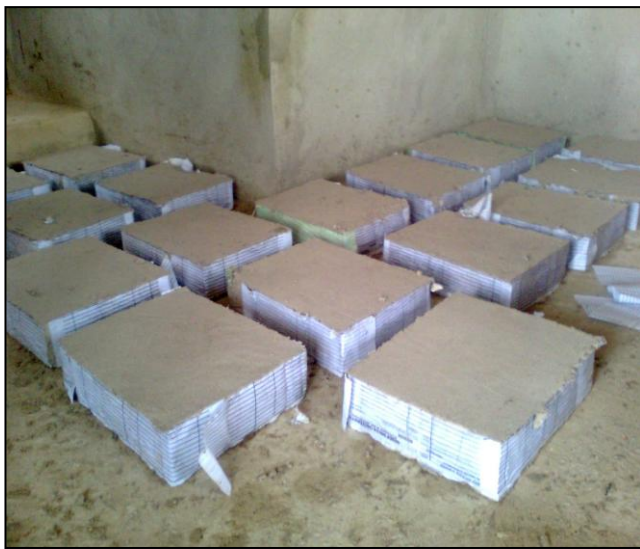
Plate 1. Insulator Bricks. These bricks are made and exposed under the shelter to dry slowly for some days to avoid cracking or warping.
