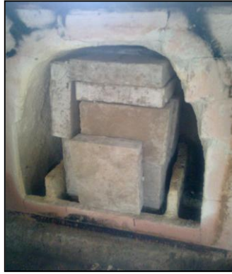
Plate 3. The insulation bricks in the kiln after firing to cone 1 (1125 °C)
