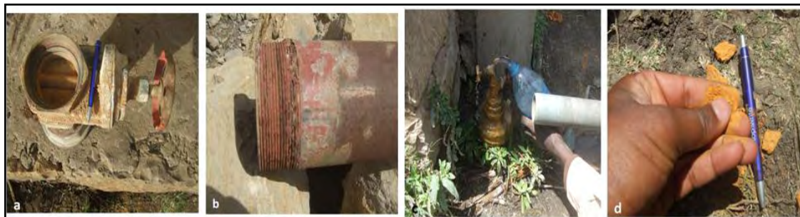
Figure 9. Selected indications of metallic pipe corrosion and scale from Mekelle City and Messebo Cement Factory water distribution systems: a) gate valve out of use, b) tread of pipe damaged, c) gate valve start to scale and rusting and d) metallic material, pipe, almost changed into soil due to corrosion.
