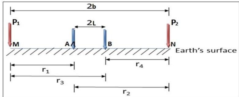
Figure 5. Schlumberger Electrodes Configuration for Reverse Switch.
