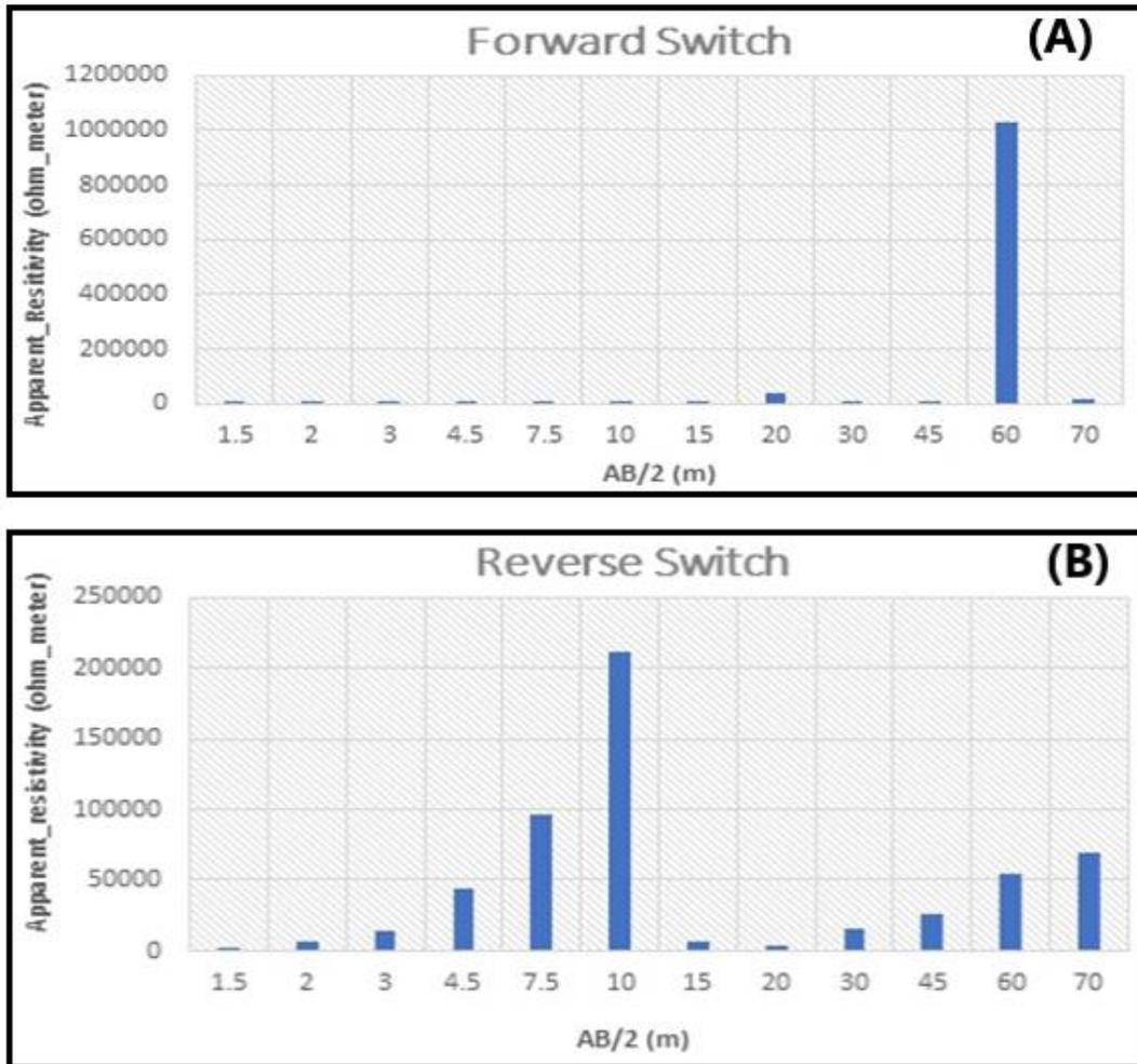
Figure 8. (a & b) displays a Stacked column relationship between forward-reverse switch configurations.
