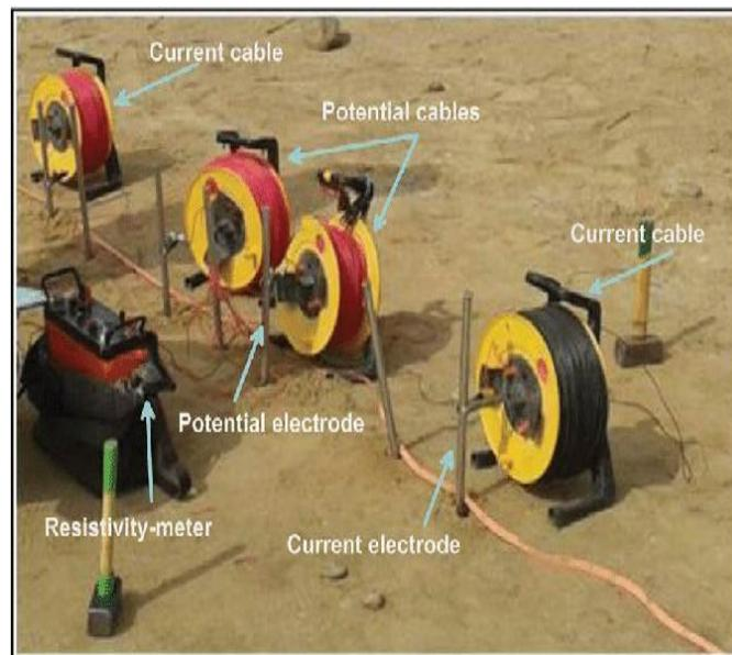
Plate I. ABEM-TERRAMETER-SAS-300C model with Accessories during the Field Work.
