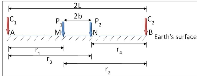
Figure 4. Schlumberger Electrodes Configuration for Forward Switch.
